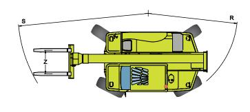
The side mounted engine ensures excellent accessibility for maintenance. Technicians can work in total safety with their feet firmly on the ground.
